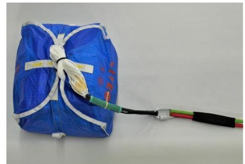
3. Insert the inner container so that the suspension lines point outwards / upwards. Let the handle run out between the container flaps 3 and 4.
