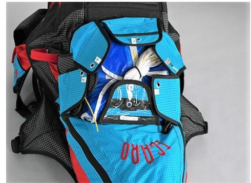
4. Close the container and remove the packing cord.
