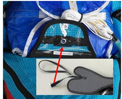
5. Insert the handle cover under the container flap 4. Place the handle cover over the container flap 3 and under the container flap 5.
