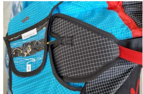
6. Insert the handle into the mount and, if necessary (according to country-specific regulations), secure with a breaking thread through both white loops (on the handle and on the harness).
