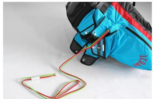
2. Loop the connection line of the reserve parachute with the connection line of the harness or connect it with a screw shackle (strength > 2400 daN). Secure connection (e.g., with neoprene tube) against slipping.
